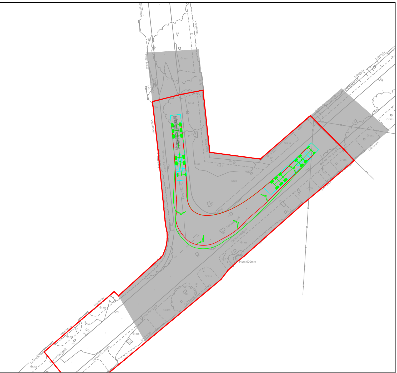
Swept Path Analysis of a 16.5m Articulated Vehicle Navigating Location U
