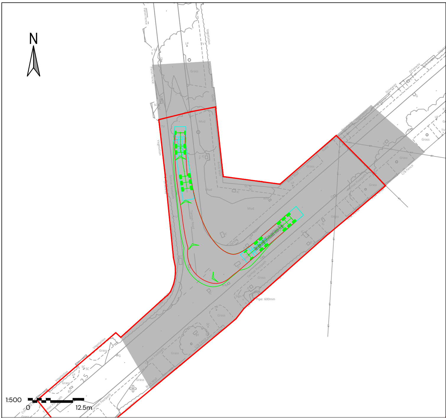
Swept Path Analysis of a 16.5m Articulated Vehicle Navigating Location U
