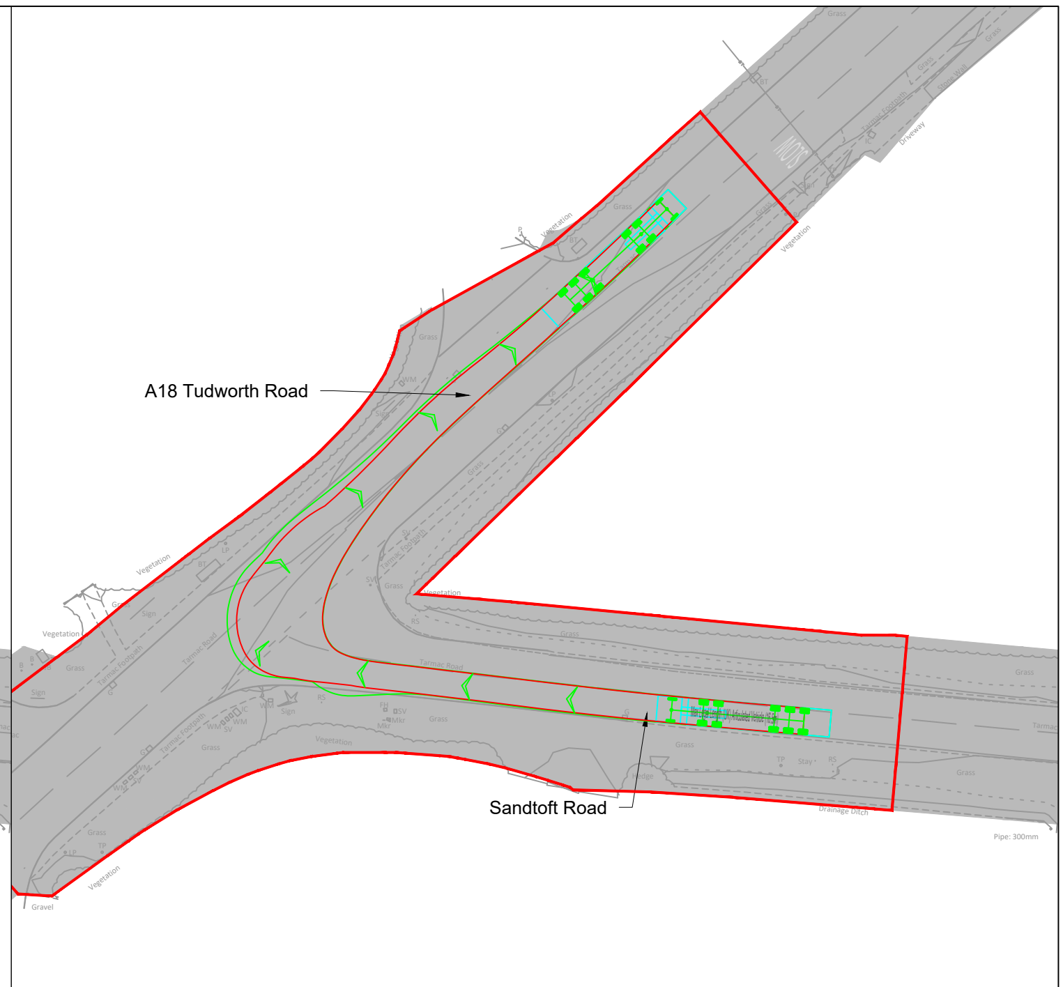
Swept Path Analysis of a 16.5m Articulated Vehicle Entering and Egressing Location G
